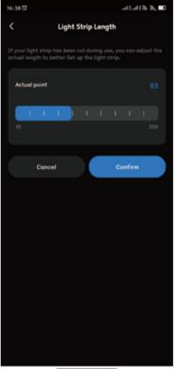
If your light has been cut during use,you can adjust the actual length to better set up the light strip.
